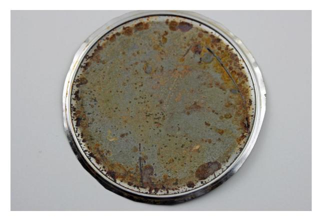
Figure 1 - Tinplate panel coated with an organic coating after OM testing in simulant B, 1 hour @  $130^{\circ}$ C + 10 days @  $60^{\circ}$ C
