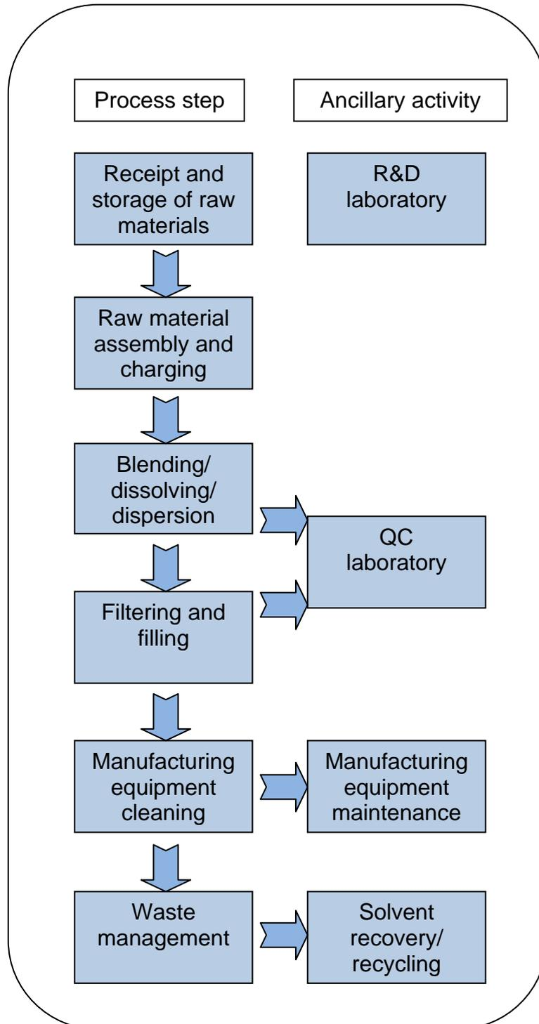
**Figure 1: coatings and inks manufacturing process steps**
