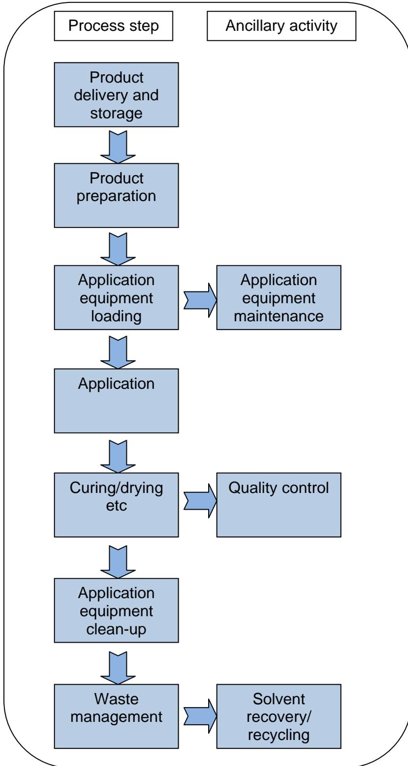
**Figure 2: coatings and inks application process steps**
