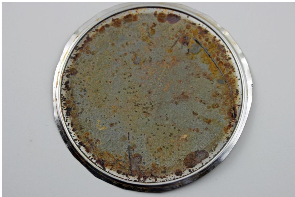
Figure 1 - Tinplate panel coated with an organic coating after OM testing in simulant B, 1 hour @ 130°C + 10 days @ 60°C
